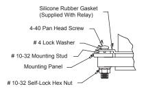
Non-Environmental Solder Termination Relay Sockets
